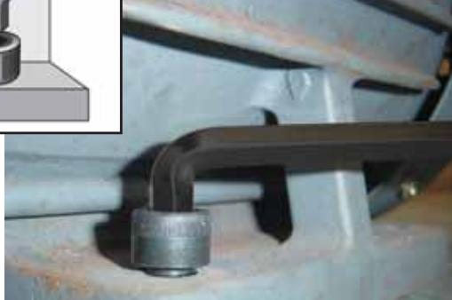
Stubby tools fit in tight spaces where there is not enough overhead clearance for a standard hex key
