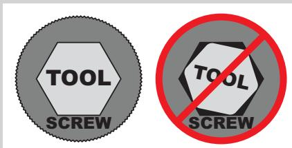
Every Bondhus tool is designed and machined to achieve an optimal fit between tool and fastener. Tools insert quickly and easily into screw head and fit snug to generate greater torque and minimize slippage and stripping.
